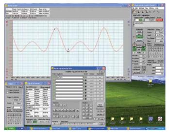
Fig.3: the maths equation builder window. We have selected to apply the equation  $X^2-X^3$  to a sinusoidal wave. The result is shown in the maths graph window. The maths graph window is a separate window that can display up to eight user-defined maths traces.
