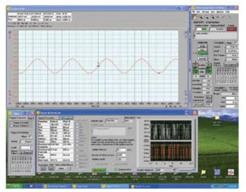
Fig.5: the signal information window, with expanded controls for data logging. This shows logging of the minimum and maximum voltage levels of the input signal. The logging rate of 10Hz is shown, as well as the instantaneous vital statistics of the analog channels.
