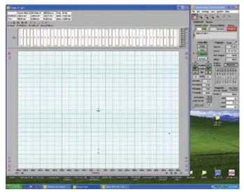
Fig.1: the scope graph window showing the digital channels. The triggering is set to a rising edge on digital channel 1. A low frequency square wave is shown, with the decoded logic values. The voltage threshold for the logic decoding can be defined.
