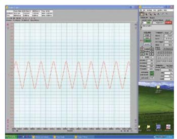
Fig.2: a relatively high frequency triangular wave shown on the scope graph using the repetitive waveform acquisition mode. The triangular wave is at a frequency around 2MHz and was generated using the optional signal generator module of the CS328A.
