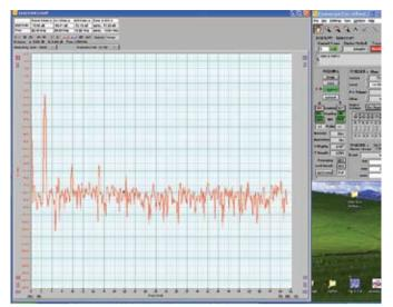
Fig.4: the Fourier Transform window is shown. The input is a low frequency waveform at around 20kHz. The small window at the top left corner inside the spectrum graph window shows information about the signals. You can choose a log plot rather than a linear one too.
